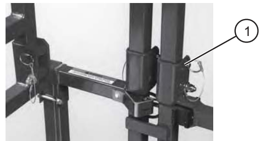
Figure 2-7. Fold-Down Guardrail System
