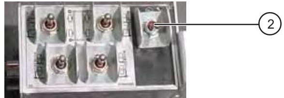
Figure 2-9B. Hydraulic Generator Control On The Auxiliary Control Box
